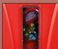
Front window for manometer inspection
